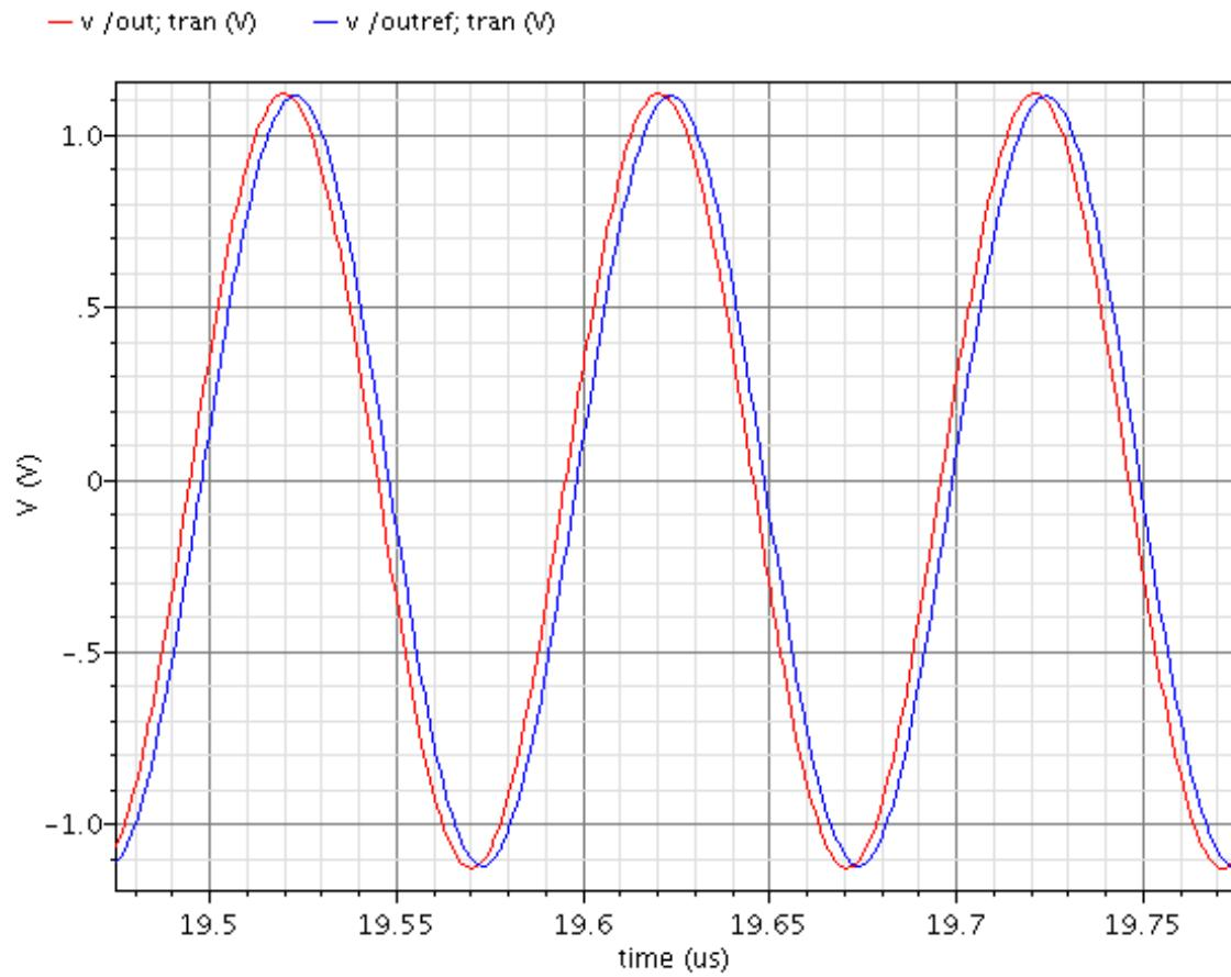
the above simulations results, show a persistent steady phase change arising from a single impulse, as required for the HL model.
