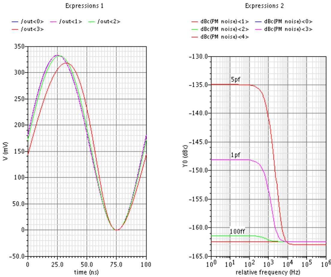
These waveforms show a dramatic up-conversion of low frequency noise, dependant on the value of load capacitor.
