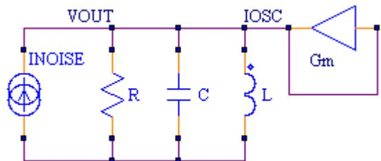
For frequencies close to the oscillator frequency, the impedance of the LCR tank is given by:
