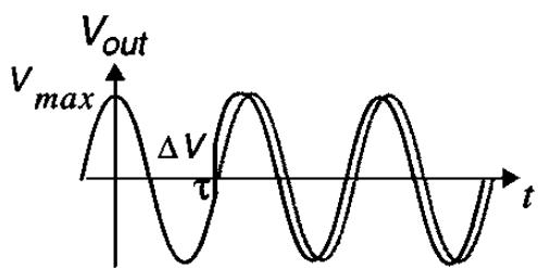
An argument is then presented that the phase of the oscillator system is, typically maximally changed near the zero crossings of the oscillator, and never changed at the oscillator peaks. It is also argued that effect of the current pulse will persist indefinitely.
