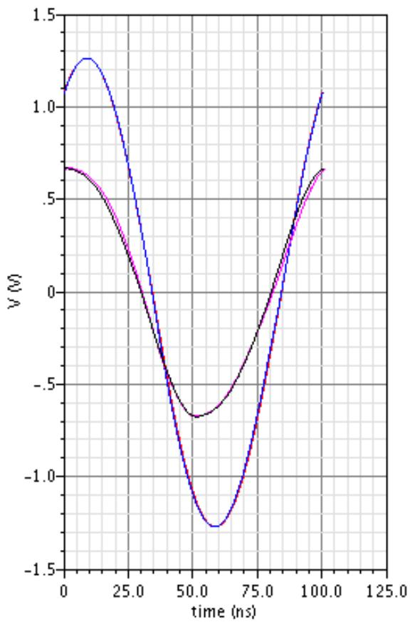
Simulations showed that with minimal non-linearity (just enough to stabilise the oscillator), up- conversion of low frequency was essentially zero. Maximum up-conversion of noise occurred at maximum square law non-linearity, and heavy diode clamping.
