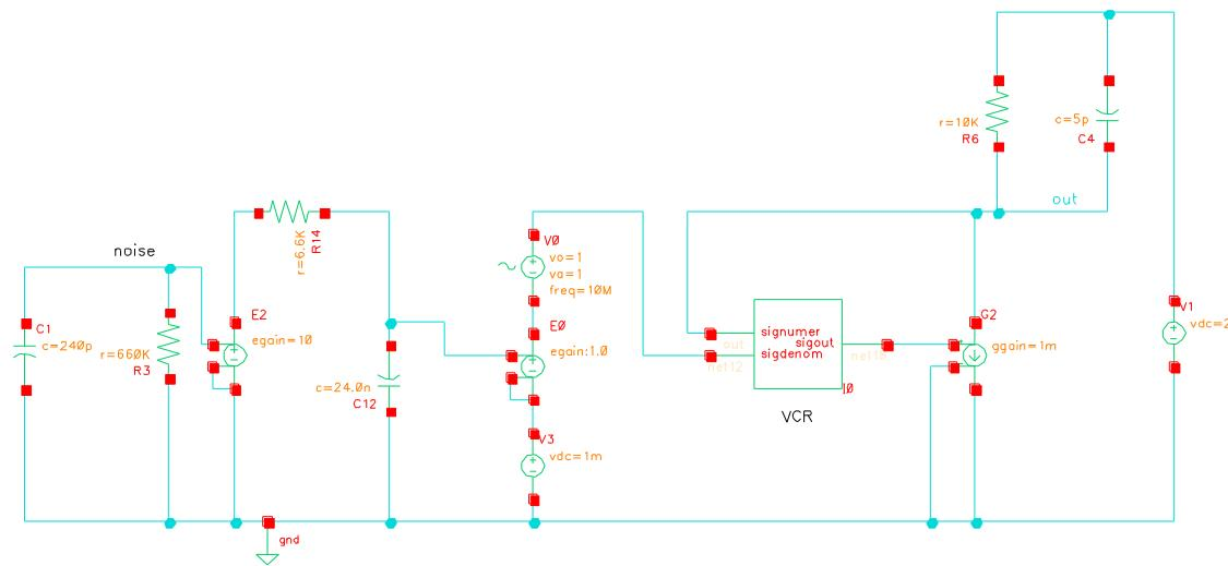
Note that this amplifier contains a fixed, linear capacitance. The block component is a divider used to construct an ideal linear VCR with a gm source. Additionally, there is a low frequency noise generator.
