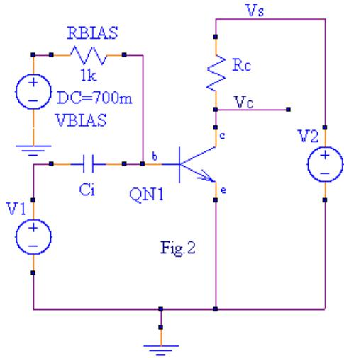
Suppose that  $R_{BIAS}$  is low enough such that its  $i_b.R_{BIAS}$  voltage drop is small.  $V_{BIAS}$  is then essentially the base emitter voltage  $V_{be}$ . From paper 1, this current is given by:
