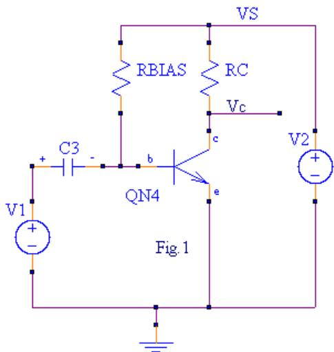
The idea here, is that Rbias feeds base current thereby producing a collector current. The ac input signal is superimposed on top of the dc Vbe via the capacitor.
