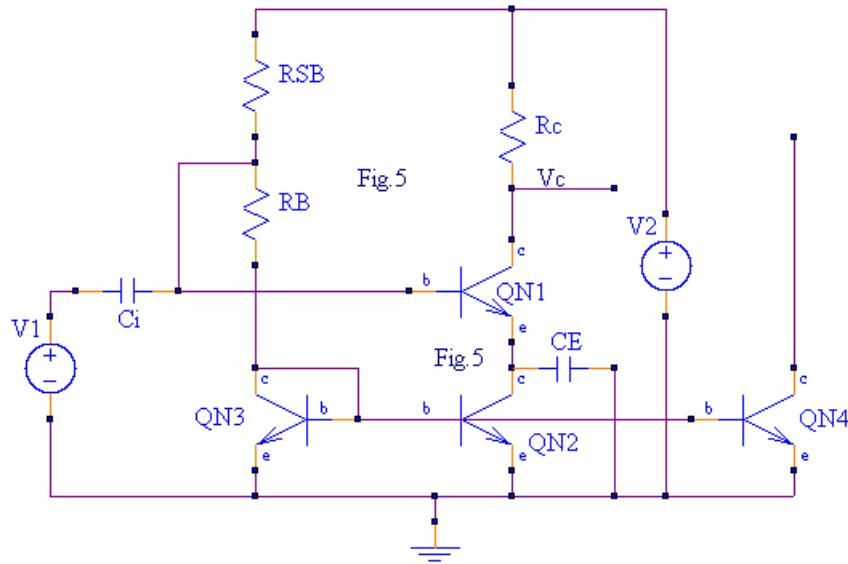
In this circuit the voltage at the base (QN1) can vary significantly without effecting the emitter/collector bias current. R<sub>SB</sub> and R<sub>B</sub> are chosen that a suitable voltage is at the base, say 1V to 2V, so long as it is less then the voltage desired at the collector, less some, to avoid bottoming (clipping).
