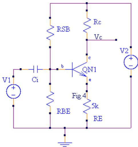
Assuming that the base current is small compared to the current through RBE, the voltage at the base node will be:
