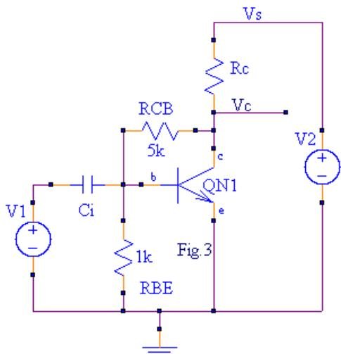
It was noted in prior papers that  $V_{be}$  only change 60mV for a 10:1 change in emitter current. i.e.  $V_{be}$  is approximately constant. If the base current in Fig.3 is a small fraction of the current through RBE, then it can be seen that RCB and RBE form a potential divider from the output collector. This means that:
